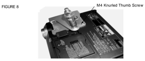
**REMINDER:** MAKE SURE TO ALLOW SUFFICIENT SLACK IN THE WIRING TO PERMIT THE PROJECTOR TO SWING DOWN ON THE HINGE TO ALLOW EASY SERVICING OF THE FILTER AND THE LAMP ASSEMBLY.
